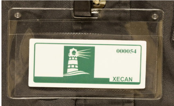
Figure 8: The XECAN patent pending lanyard can be reliably detected by the RFID readers in clinics. It has a very small form factor (1.2”X2.1”)
